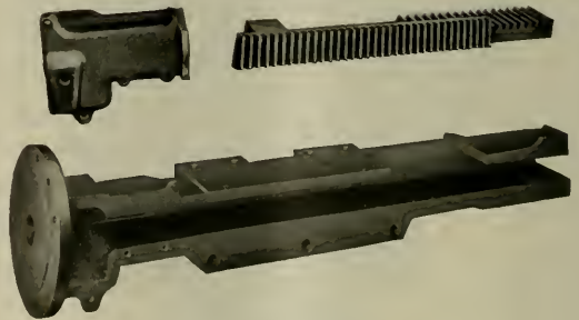
RACK AND RACK HOUSING DISMANTLED
